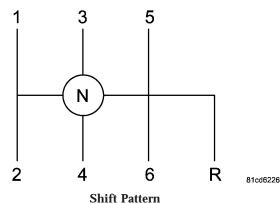
Fully depress the clutch pedal before shifting gears. As you release the clutch pedal, lightly depress the accelerator pedal.
